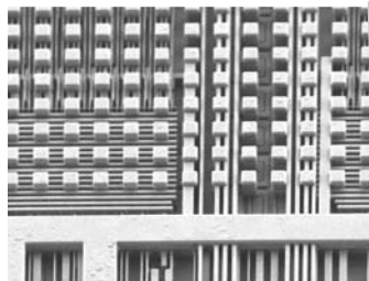
Failure analysis - fast metal layer exposure in the PlasmaPro NGP FA ICP
